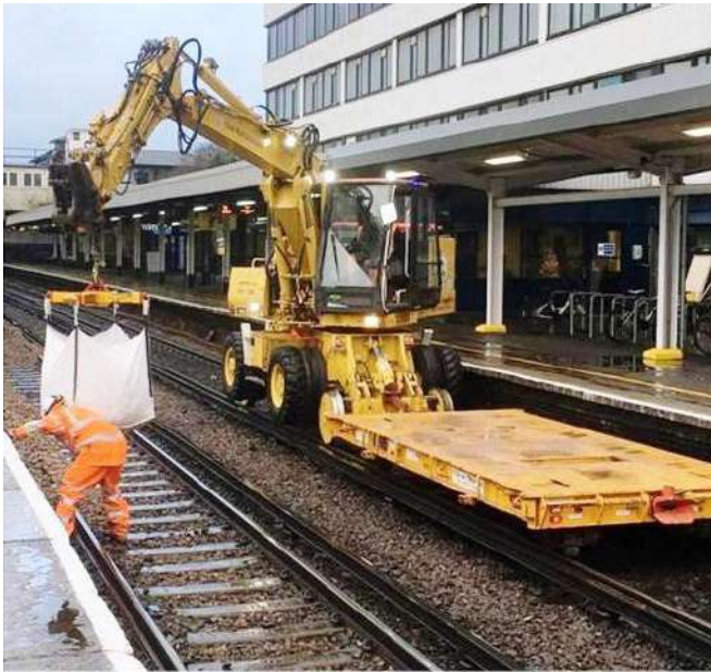
Suprailer/CASE 988 with p-way trailer at work on the Big Railway Photo : TRS
